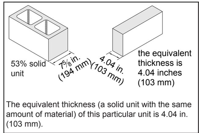
**Figure 1—Equivalent Thickness**
