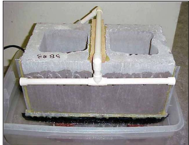
**Figure 2—Specimen Undergoing the Spray Bar Test Method**
