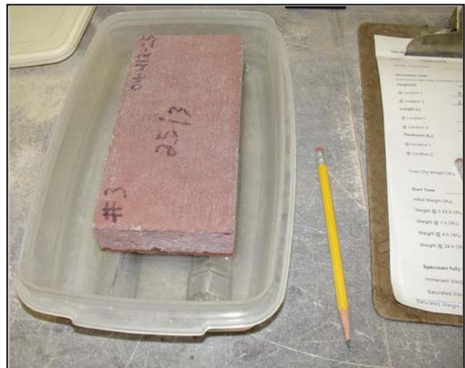
**Figure 3—Specimen Undergoing the Water Uptake Test Method**
