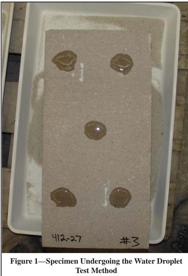
**Figure 1—Specimen Undergoing the Water Droplet Test Method**
