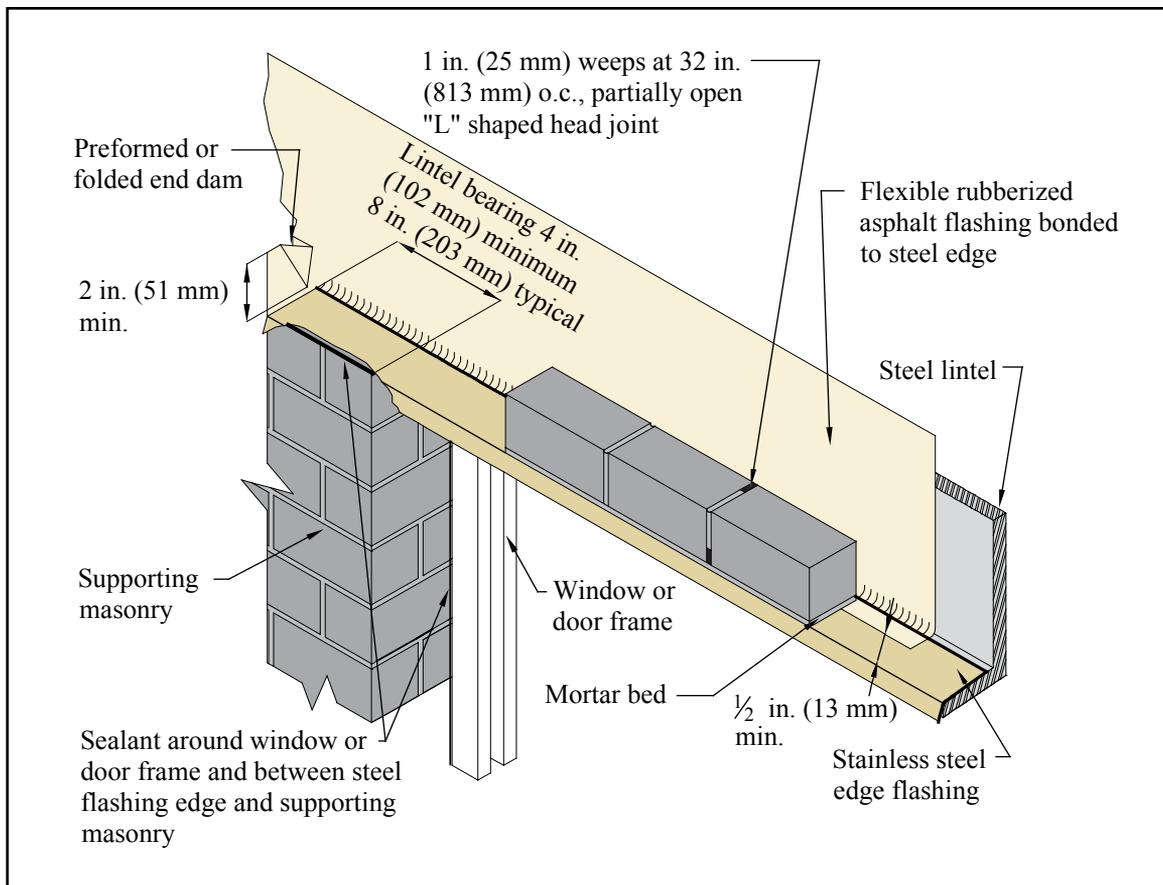
**Figure 2—Steel Lintel Flashing Detail (ref. 8)**
