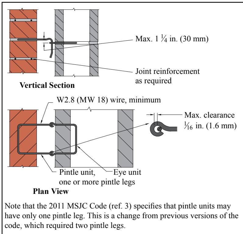
**Figure 3—Adjustable Anchors**
