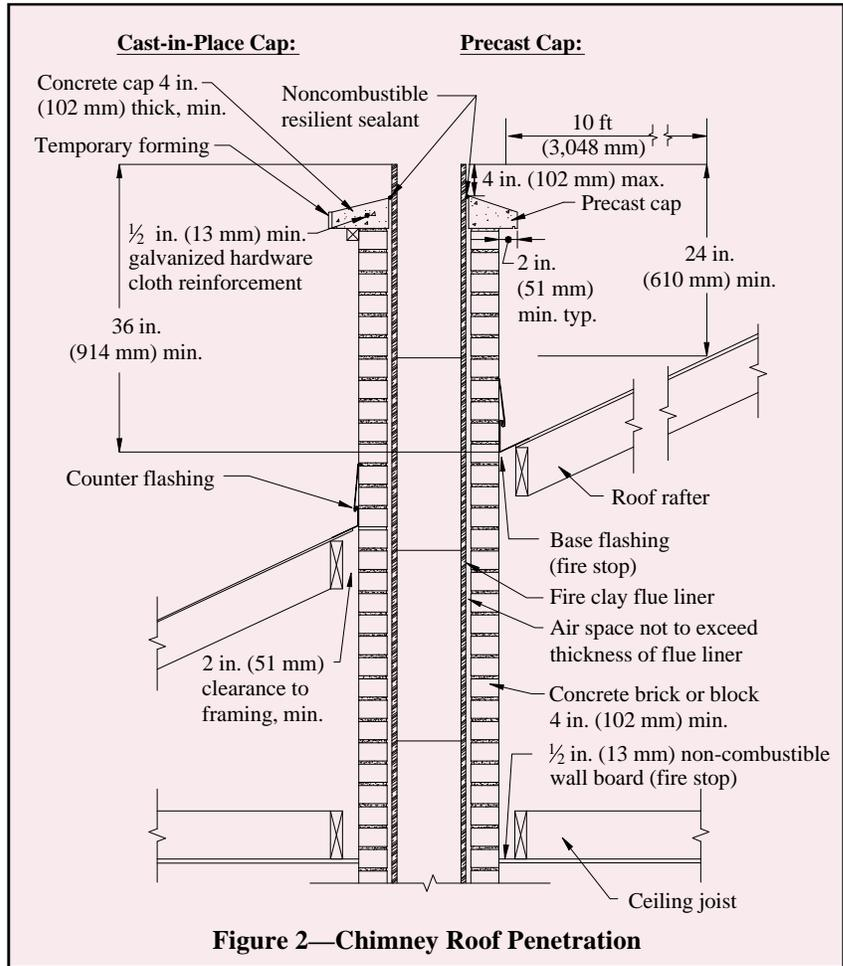
**Figure 2—Chimney Roof Penetration**
