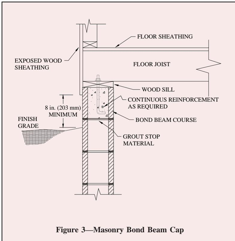
Figure 3—Masonry Bond Beam Cap
