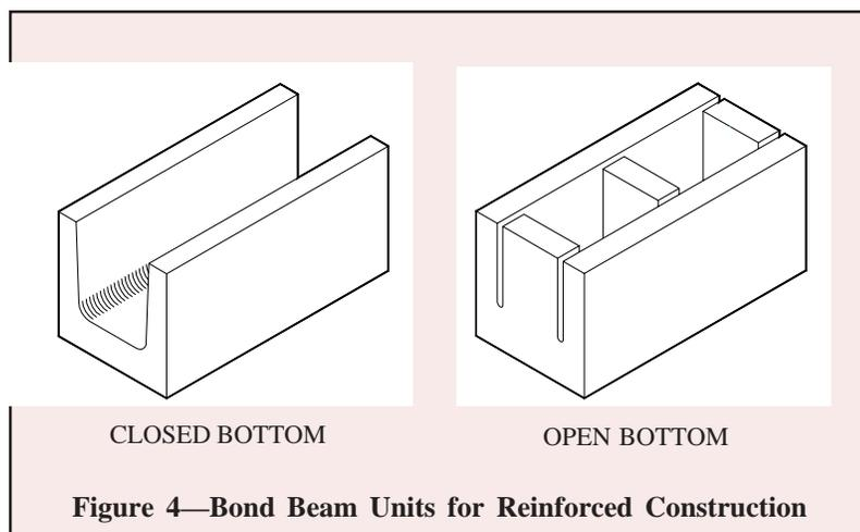
Figure 4—Bond Beam Units for Reinforced Construction
