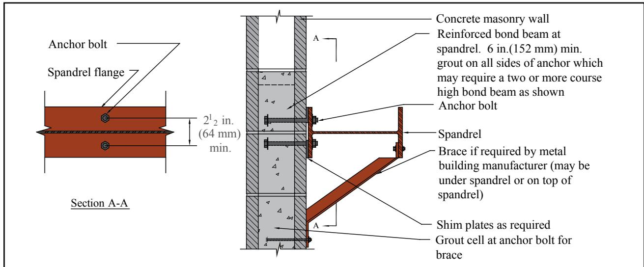
**Figure 6—Structural Spandrel for Lateral Load Detail**
