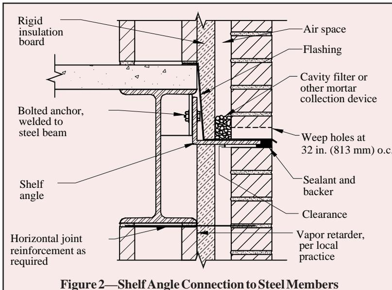
Figure 2—Shelf Angle Connection to Steel Members
