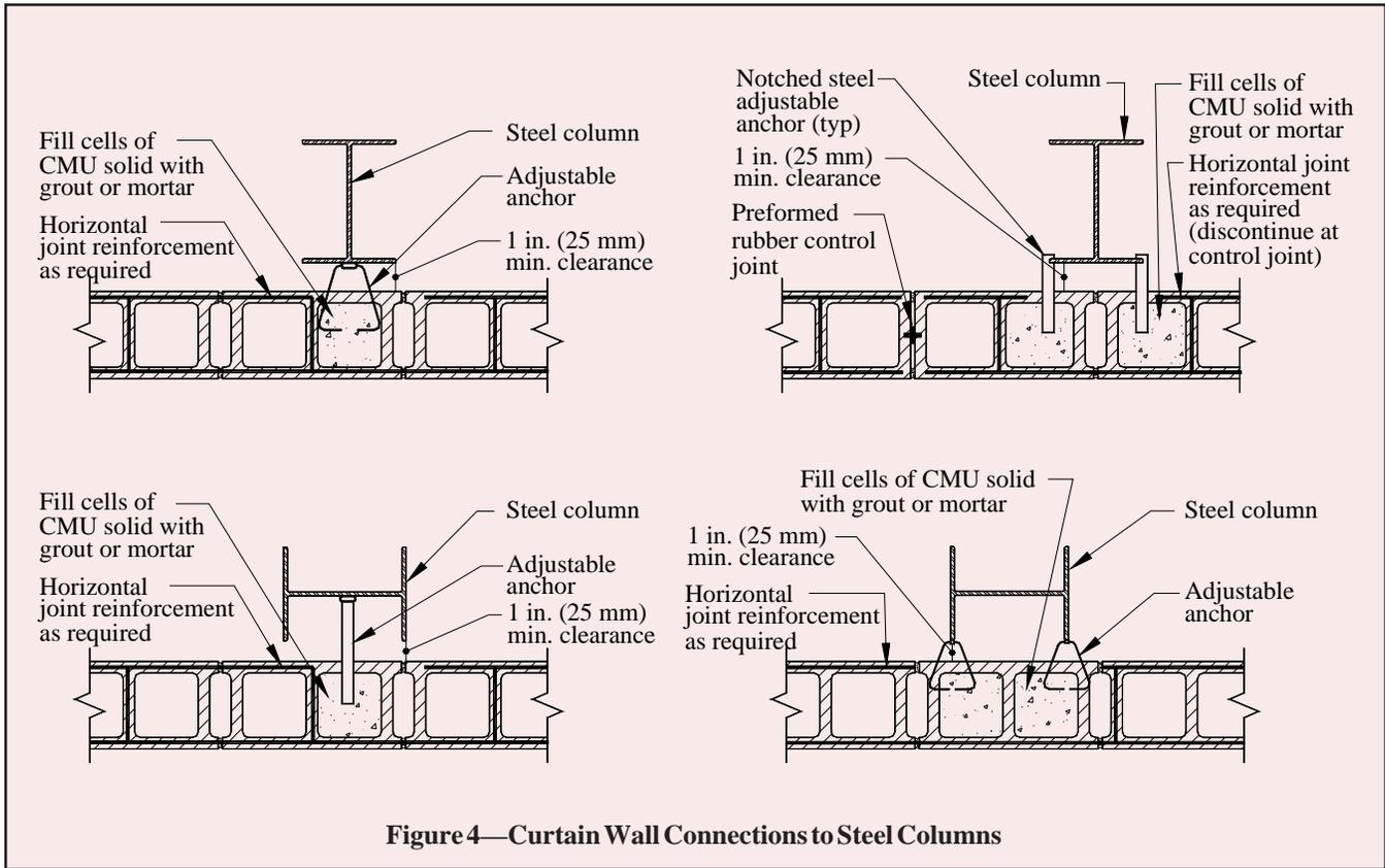
Figure 4—Curtain Wall Connections to Steel Columns
