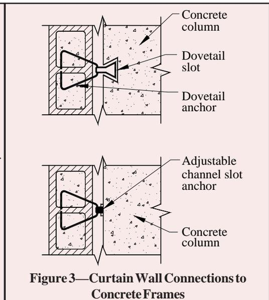
Figure 3—Curtain Wall Connections to Concrete Frames
