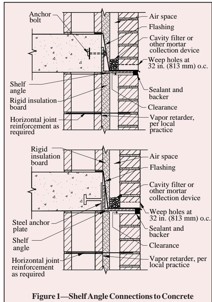
**Figure 1—Shelf Angle Connections to Concrete**
