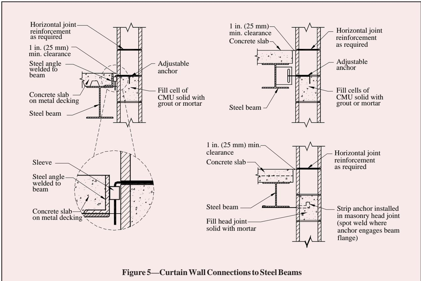
Figure 5—Curtain Wall Connections to Steel Beams
