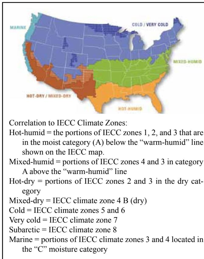
Figure 1— Condensation Control Climate Zones (ref. 4)
