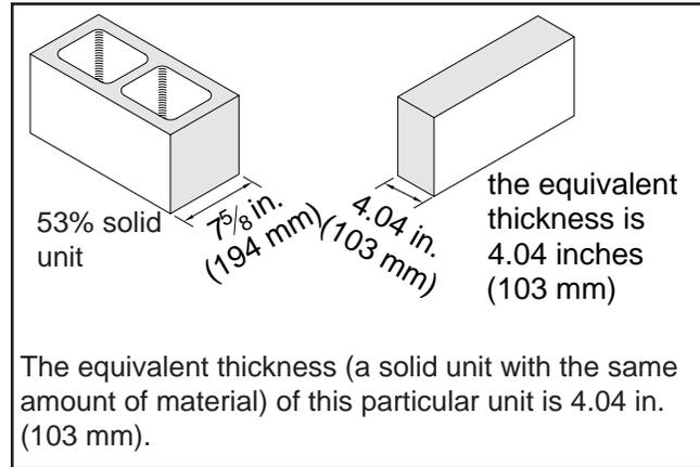
**Figure 1—Equivalent Thickness**
