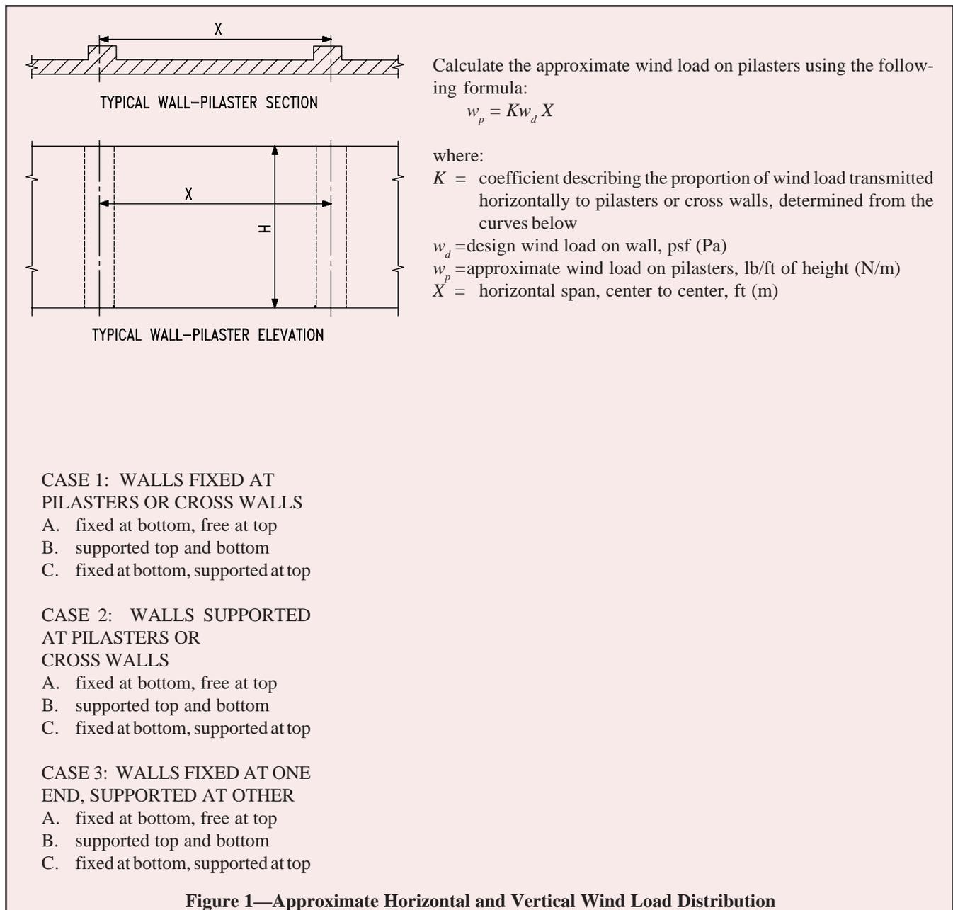
Figure 1—Approximate Horizontal and Vertical Wind Load Distribution
