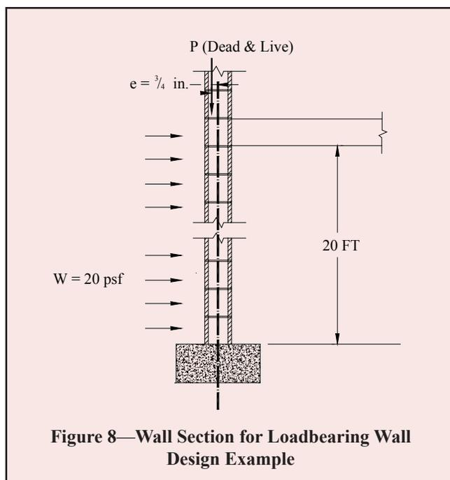
Figure 8—Wall Section for Loadbearing Wall Design Example
