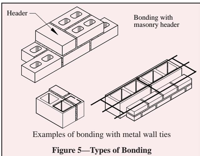
**Bonding with metal wall ties (other than adjustable ties).**
