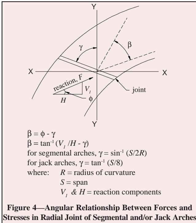
**Figure 4—Angular Relationship Between Forces and Stresses in Radial Joint of Segmental and/or Jack Arches**
