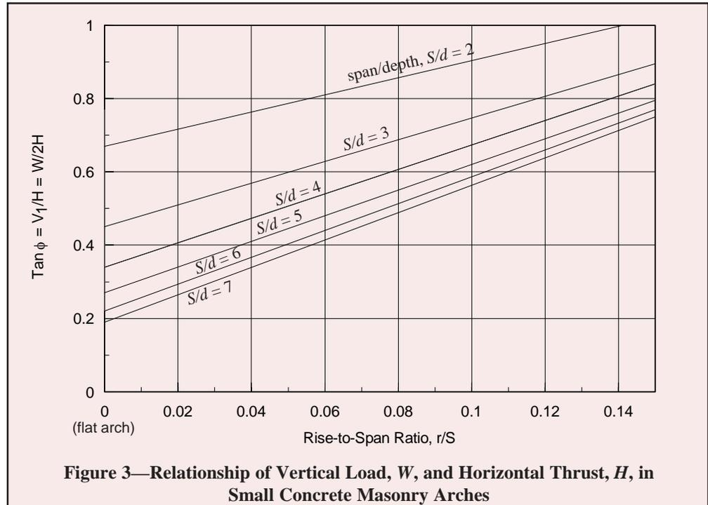
**Figure 3—Relationship of Vertical Load,  $W$ , and Horizontal Thrust,  $H$ , in Small Concrete Masonry Arches**
