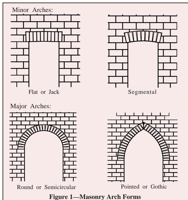
Figure 1—Masonry Arch Forms
