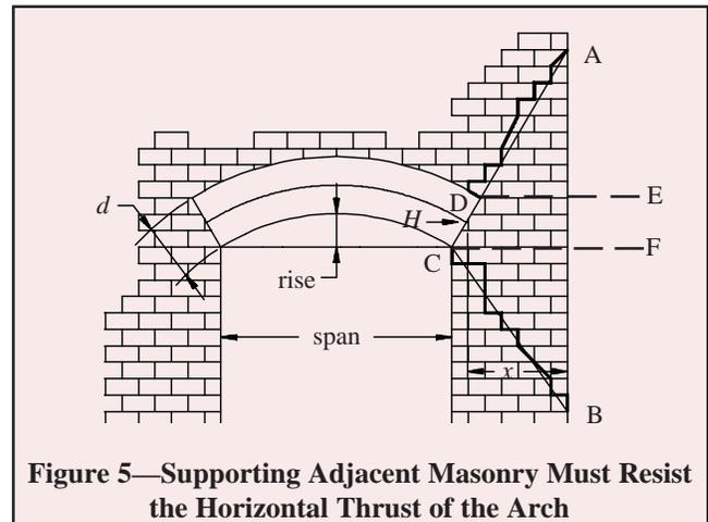
**Figure 5—Supporting Adjacent Masonry Must Resist the Horizontal Thrust of the Arch**
