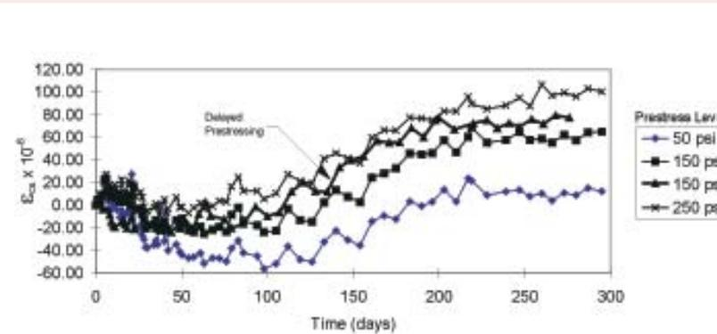
Figure 5—Creep Strain for Lightweight, 1580  $f'_{mt}$  Specimens (ref. 1)
