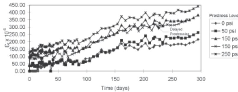
Figure 3—Total Strain for Lightweight, 1580  $f'_{mt}$  Specimens (ref. 1)
