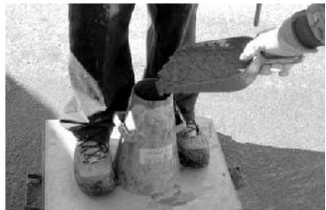
Figure 1—Filling the Slump Cone
